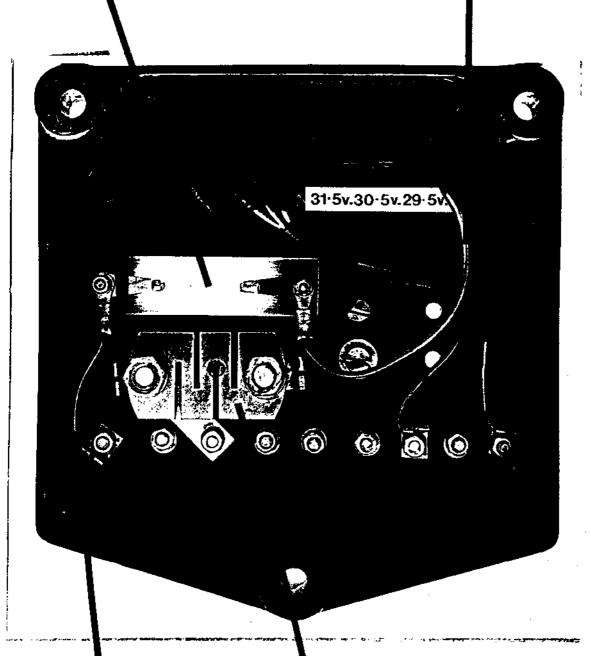
SHORT LEAD D+ TO RESISTOR SHUNT
